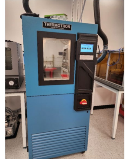
A cryogenic chamber will be used in the B-LO Zero project's battery material testing. Photo courtesy Nick Rolston/ASU
