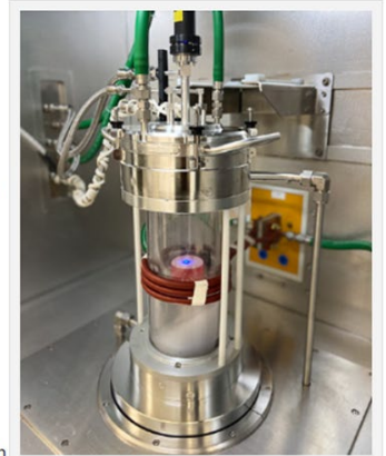
A metal-organic chemical vapor deposition, or MOCVD, reactor from Agnitron used by Nidhin Kurian Kalarickal in his gallium oxide etching research. Photo courtesy of Nidhin Kurian Kalarickal/ASU
